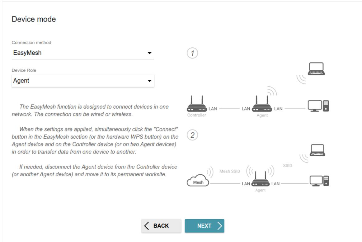
Figure 45. Configuring the EasyMesh function for a subordinate device.
