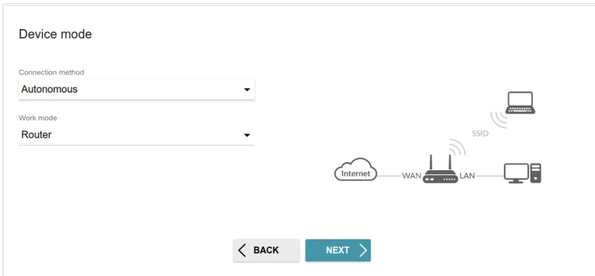
The screenshot shows a web interface titled "Device mode". It contains two dropdown menus: "Connection method" with "Autonomous" selected, and "Work mode" with "Router" selected. To the right is a diagram of a router connected to an "Internet" cloud via a "WAN" port, and to a laptop and a PC via "LAN" and "SSID" wireless connections. At the bottom are two buttons: a grey "BACK" button with a left arrow and a blue "NEXT" button with a right arrow.
