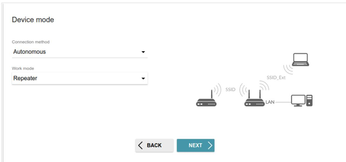
Figure 40. Selecting an operation mode. The **Repeater** mode.
