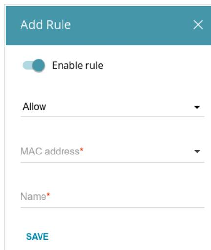
Figure 132. The window for adding a rule for the MAC filter.
