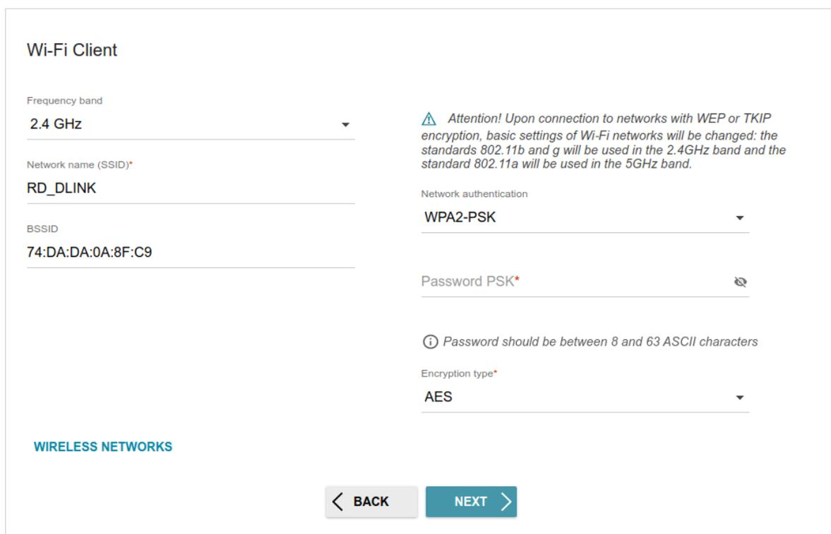
Figure 49. The page for configuring the Wi-Fi client.
