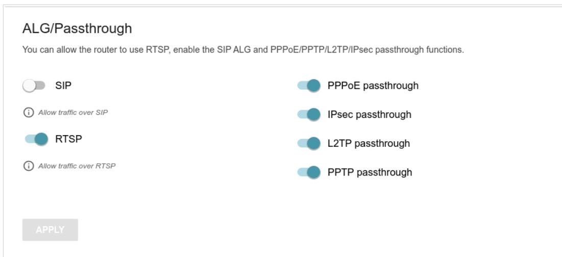
Figure 164. The **Functions / Advanced / ALG/Passthrough** page.
