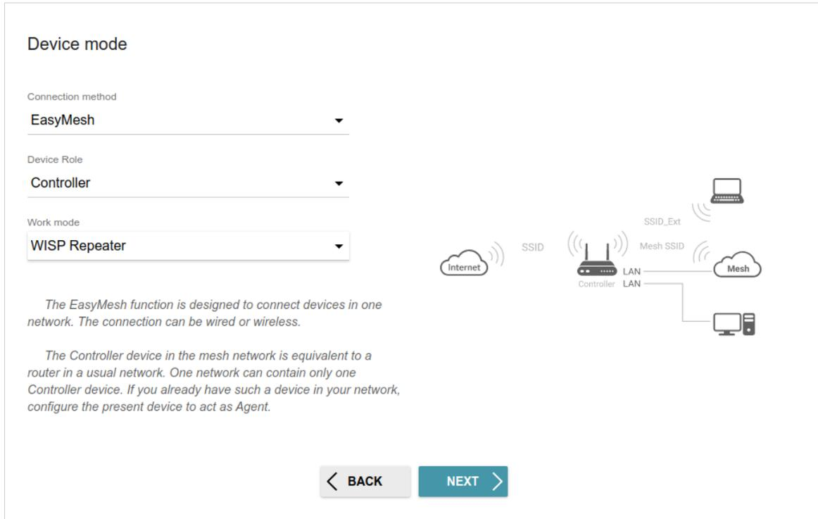
Figure 44. Configuring the EasyMesh function for a main device. The **WISP Repeater** mode.
