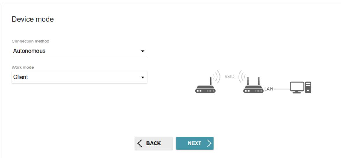
Figure 41. Selecting an operation mode. The **Client** mode.
