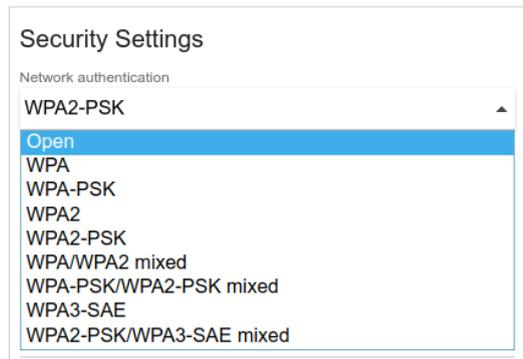
Figure 94. Network authentication types supported by the router.
