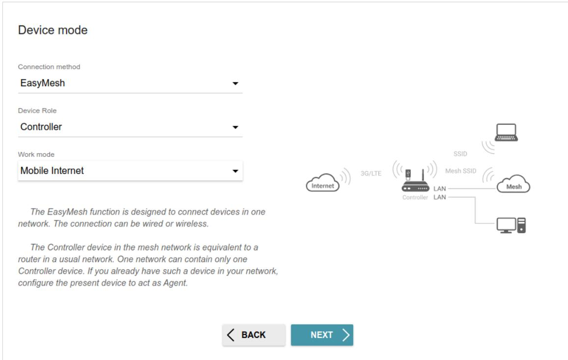
Figure 43. Configuring the EasyMesh function for a main device. The **Mobile Internet** mode.
